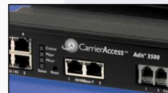
Adit 3500 SIP to PRI Trunk Gateway and Router
